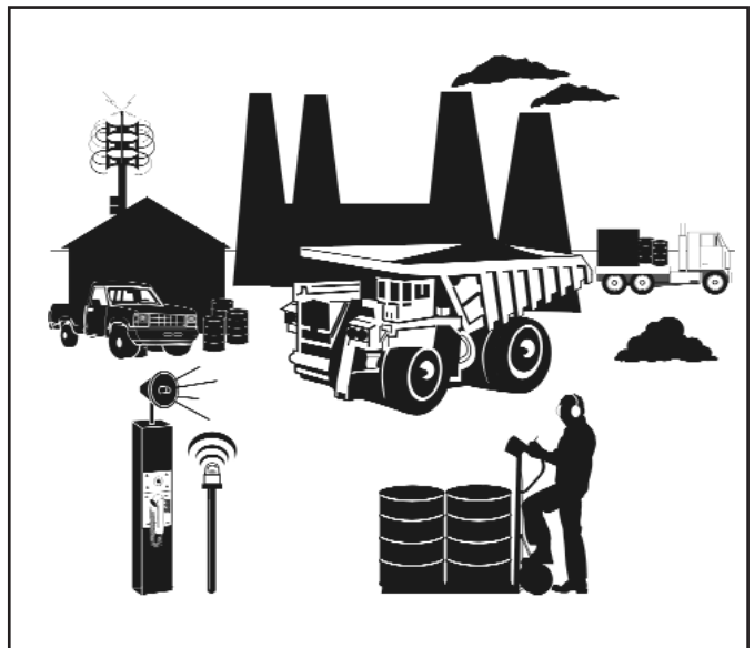
Figure 4. Acceptable solution: Tower signaling system integrated with distributed loudspeaker and/or visual indicators enhance employee awareness.
